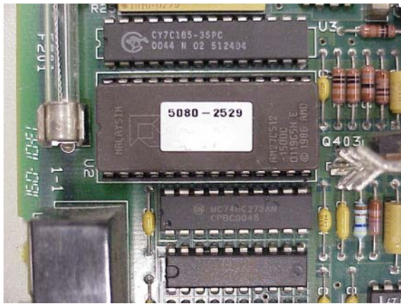
FIGURE 1 Tested PCA P/N 66101-61022 (Location of Circuit Reference “U2”)
